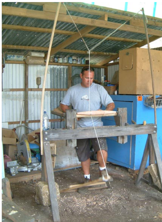
This is a simple but effective lathe, powered by a strong leg, using a springy sapling as resistance on the turn.
